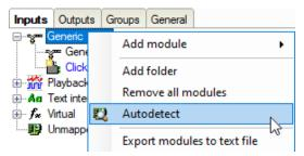
By applying Autodetect, a *Generic Unicast UDP* module with 32 analog signals (data type FLOAT) and 32 digital signals is created for each link.
