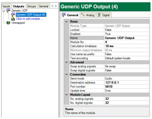
The parameters are almost identical to those of the input module, see **7** General module settings, page 12.
